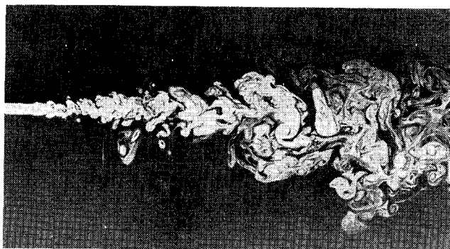
Fig. 8 Laser-induced fluorescence visualization of an axisymmetric jet. 47
